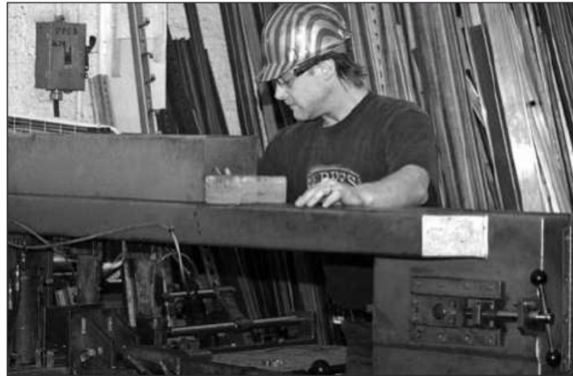
Eberl Iron Works employee Jeffery Ersing operates a saw to cut Unistrut metal framing for a future job.
